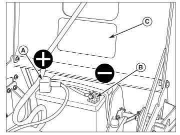
Figure 2. Connect the Battery
